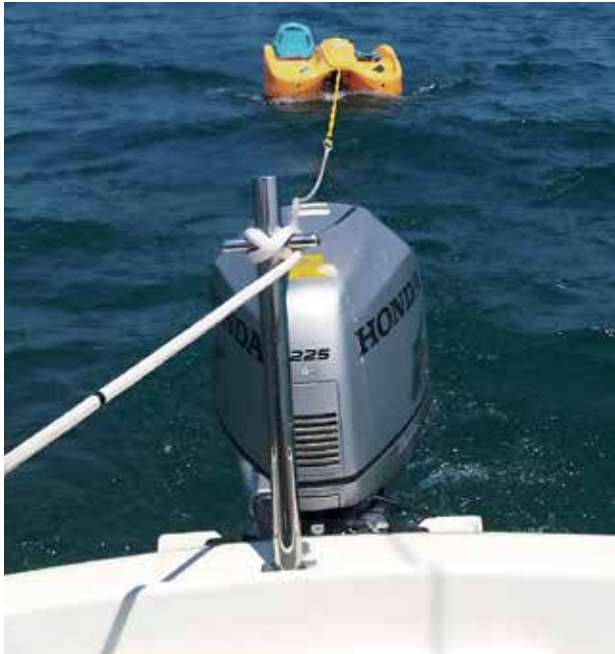
TOWLINE CONNECTION SHOWING BRIDLE ANGLE
