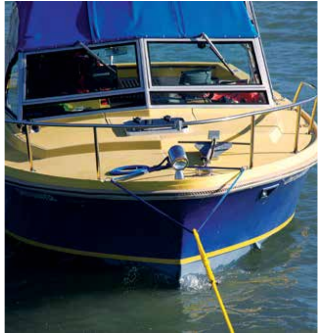
TOWLINE CONNECTION SHOWING BRIDLE ANGLE
