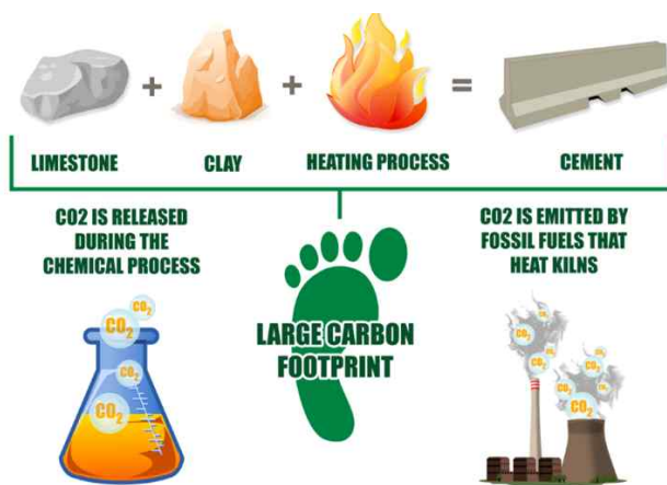
Figure 28. Cement product process
